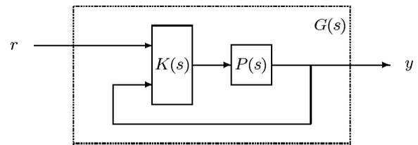
Fig. 1 Block diagram of SISO system.
